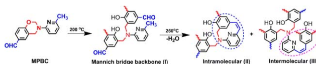
Scheme 2. Ring-opening polymerization and Knoevenagel reaction of MPBC upon curing. [Color figure can be viewed in the online issue, which is available at wileyonlinelibrary.com .]
